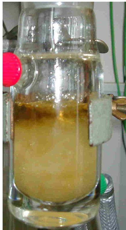
Fig. 3: Static layer crystallization
