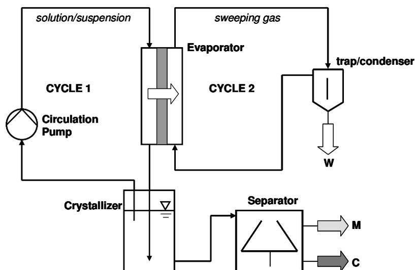
**Figure 1:** Schematic representation of the membrane based crystallization setup
