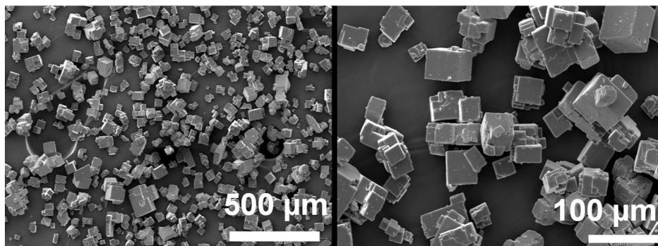
**Figure 3:** REM-micrographs of the produced NaCl crystals
