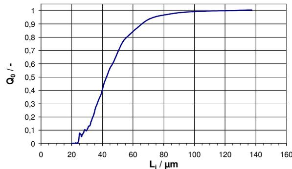
**Figure 4:** Representative particle size distribution of the produced NaCl crystals
