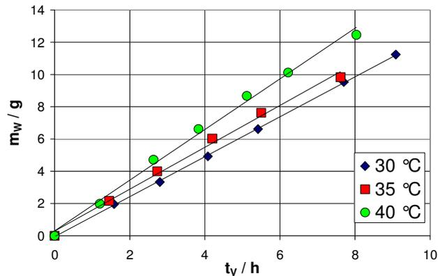
**Figure 2:** Mass of transmembrane evaporated water in dependence of the experimental time
