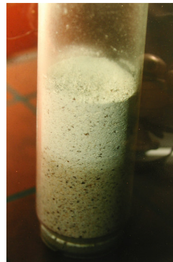
Crushed almonds with leached zone at the top after the extraction with CO 2 in a fixed bed
